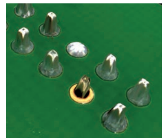
Insufficient wetting (front) and missing pin (back)
